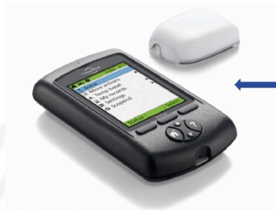
Modified Omnipod insulin pump BLE relay
